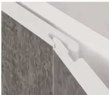
4、对齐锁扣拼接 4. Align and lock the joints
