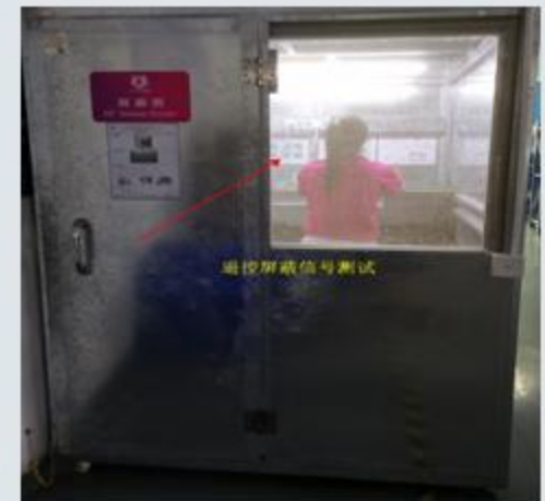
RF Shield Room
