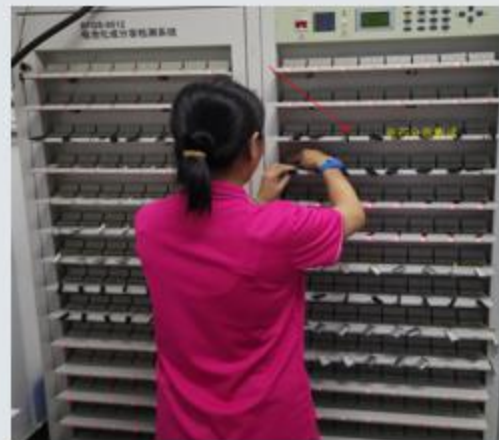
Battery Capacity Test
