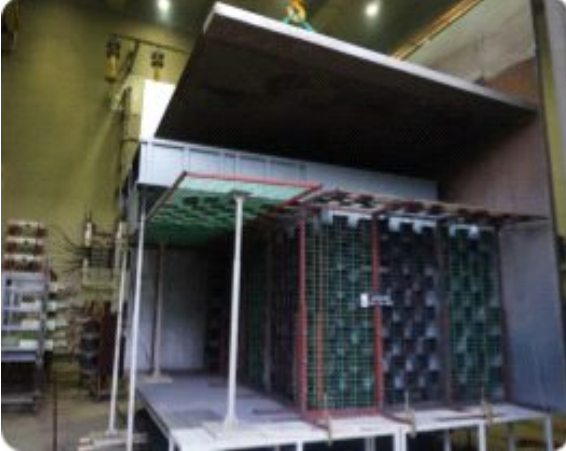
Internal arcing faults test
