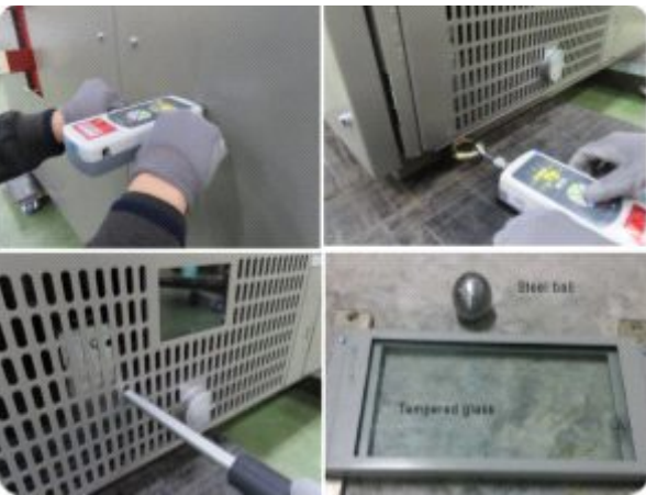
Enclosure and ventilation opening test
