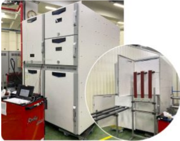
Rated continuous current tests (Temperature rise test)
