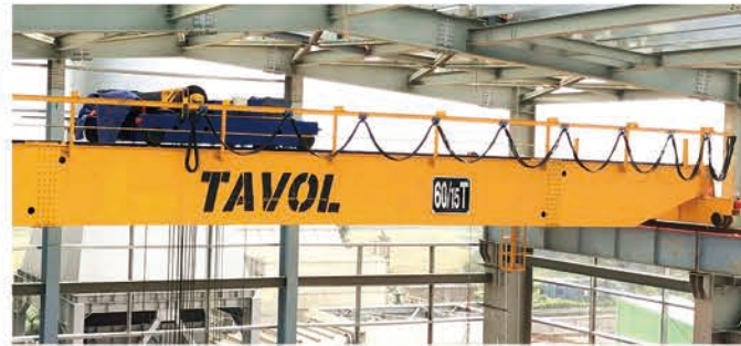
双梁桥式起重机 Double Girder Overhead Crane
