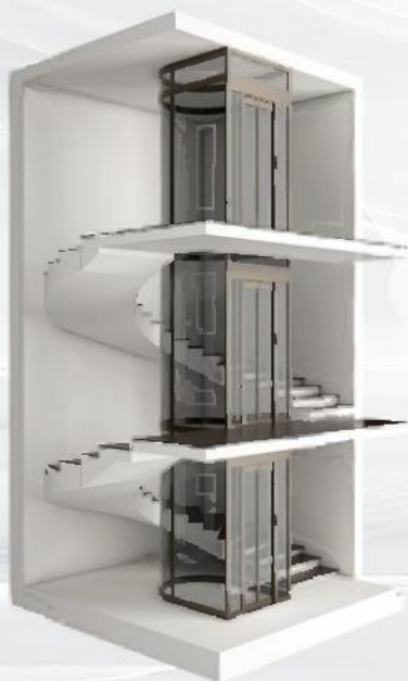
Semi-circular three- quarter-turn stair
