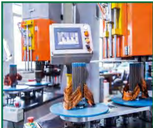
coil wire winding
