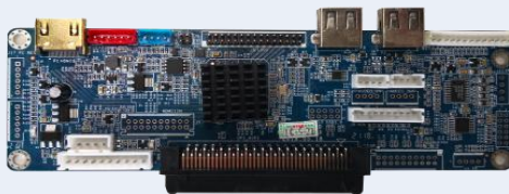
Support LVDS dot screen 1080P+15W amplifier+HDMI IN+VGA IN
