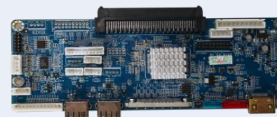
Support Vbyone dot screen 4K 120HZ+15W amplifier+HDMI IN+VGA IN
