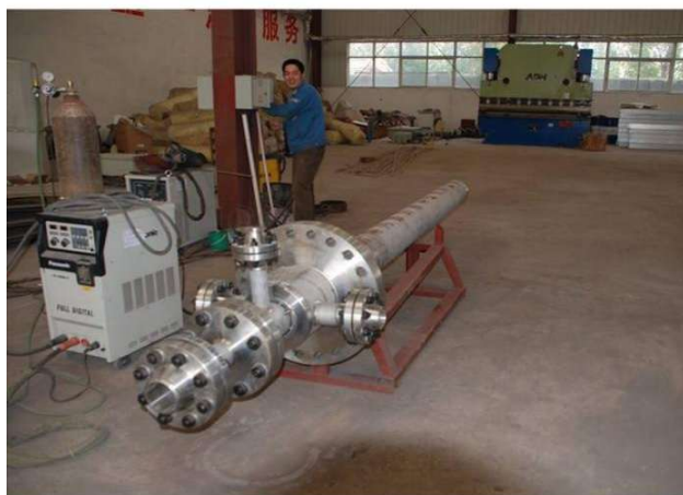
转窑燃烧器 Rotary kiln burner
