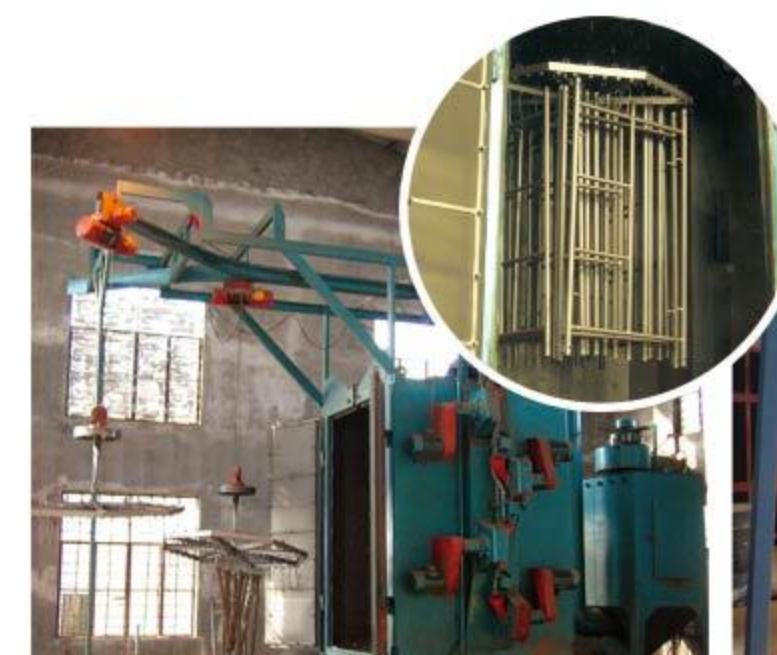
喷砂处理设备 Sandblasting treatment equipment
