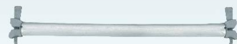
RFH-B005B 横杆(mm) Aluminium Alloy Ring Lock Scaffolding Ledger 732 1088 1400 1572 2072 2572 3072 Φ48.3x4mm
