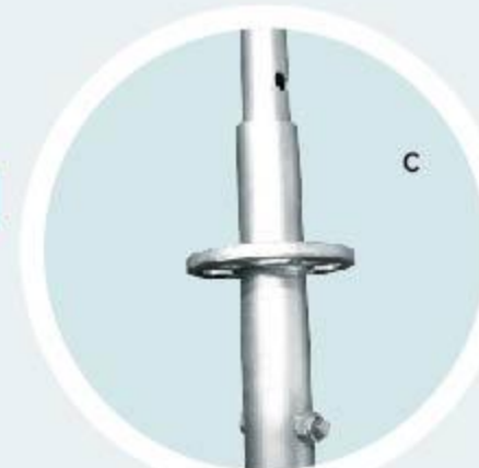
RFH-B001A(mm) 立柱 Standard 500 1000 1500 2000 2500 3000 4000 Φ48.3×3.25mm Φ60.3×3.5mm
