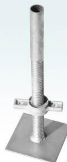
RFH-B011J 调节底座 Jack Base 450mm Φ 32mm 150x150x5mm
