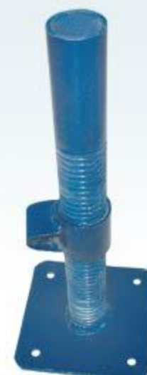
RFH-B011E 空心调节底座 Hollow Screw Jack Base 600,914,1524 mm Φ 40x4mm 140x140x5mm
