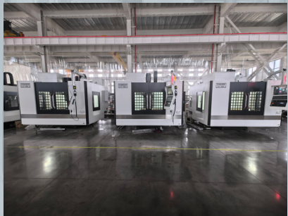
6 units EV1160A with FANUC 31i
