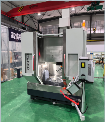
2 units DX650 with Siemens one
