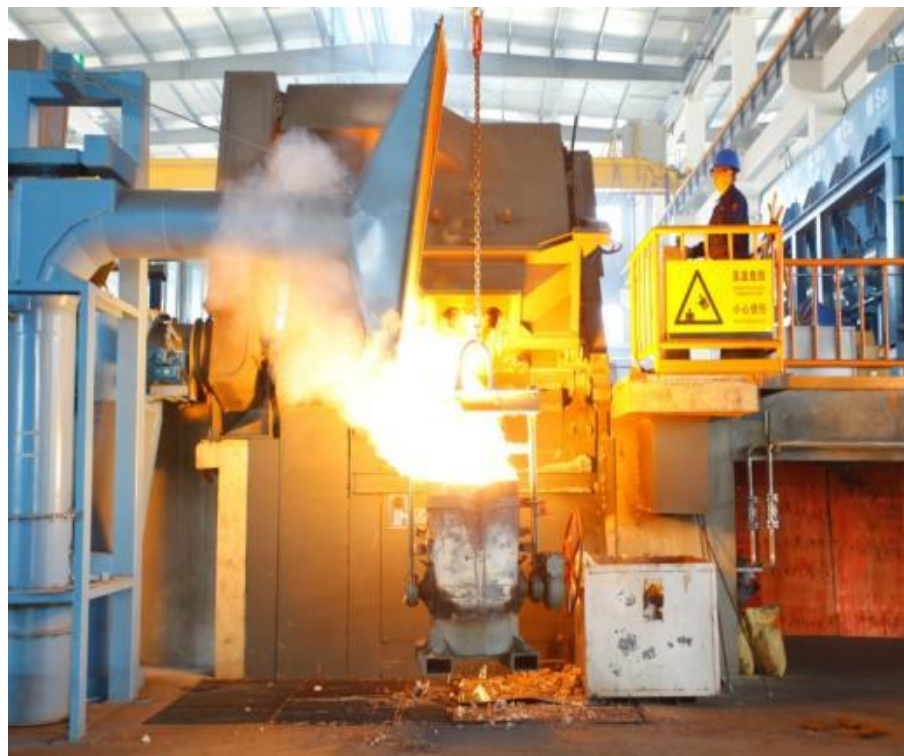
2台5T应达感应电炉 Two 5T Inductotherm Induction Electric Furnaces
