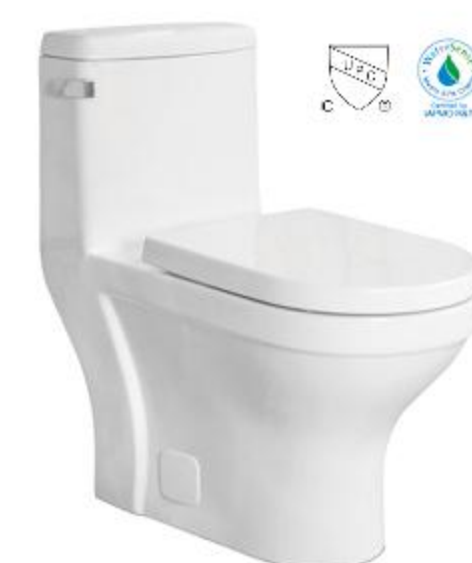
FTO-8004 Siphonic One-piece toilet Size: 700×364×750mm S-trap, 305mm Roughing-in
