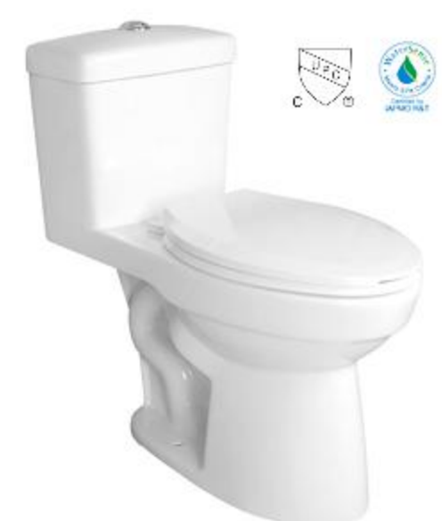
FTO-8848 Siphonic One-piece toilet Size: 720×367×740mm S-trap, 305mm Roughing-in
