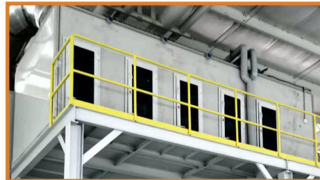
自循环供风 Recirculating Air Supply
