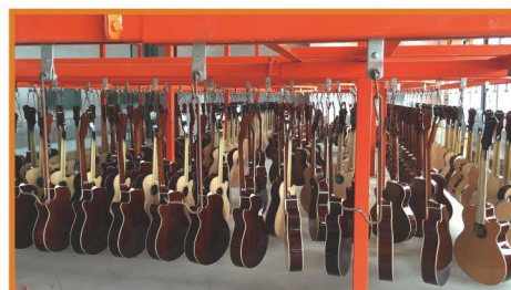
吊挂线流平干燥区 Overhead Conveying Line Flash Off And Drying Area
