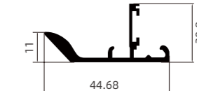
FY-A100 卡 5 厘免开铰链孔拇指拉手 Snap-on 5mm Hinge Hole-Free Thumb-style Pull Handle.
