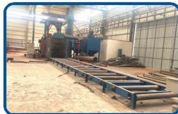
抛丸除锈 Shot blasting for rust removal
