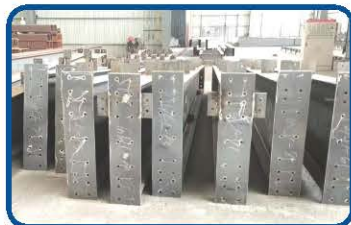
打磨前质检 Quality inspection before blasting
