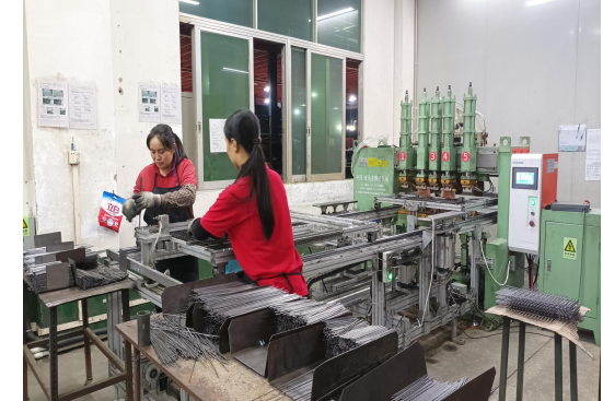
Gantry spot welder*1
