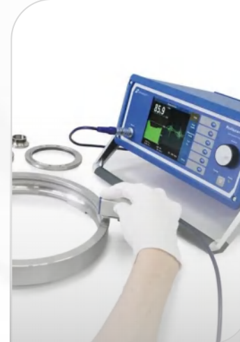
Barkhausen Rollscan350 noise analysis-grinding burn
