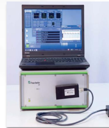
Fraunhofer Nondestructive Test of case depth and hardness
