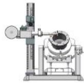
Pipe-flange internal fillet welding
