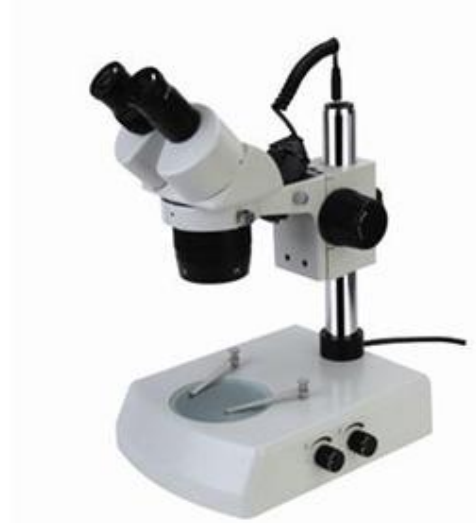
XT24 Stereo Microscope (with up and down LED illumination)
