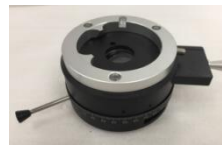
Analyzer Unit & Bertrand Lens
