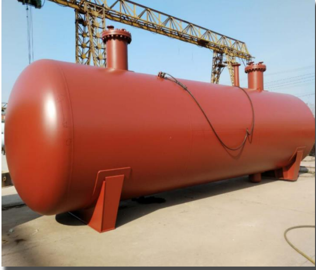
Buried storage tank
