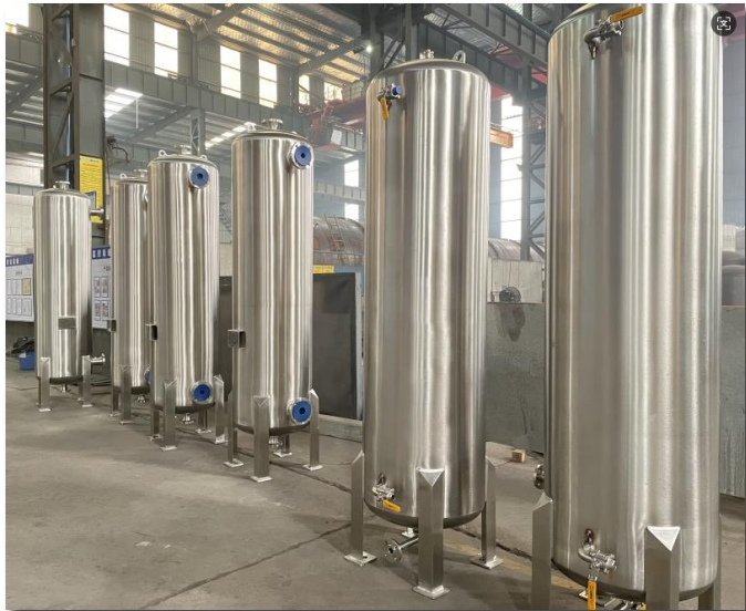
ASME and NR-13 certified stainless steel exchangers
