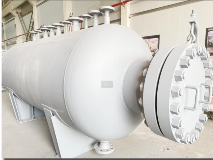
Liquid chlorine vaporizer
