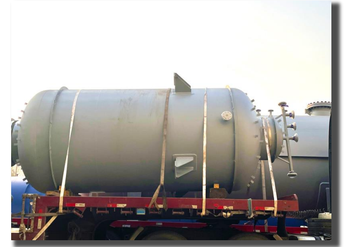
Liquid chlorine vaporizer
