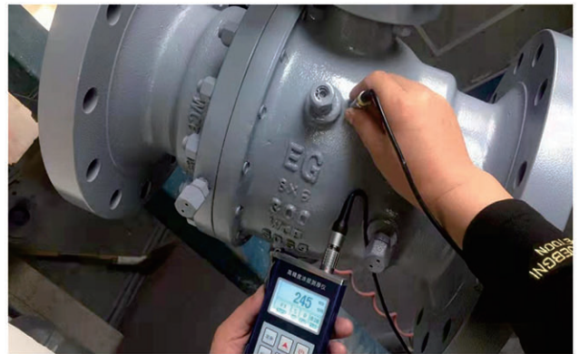
Paint Thickness Inspection
