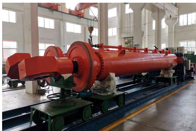
福建永泰抽水蓄能电站 QPKY-1250/5000kN-6.4m 4套 Fujian Yongtai Pumped Storage Power Station
