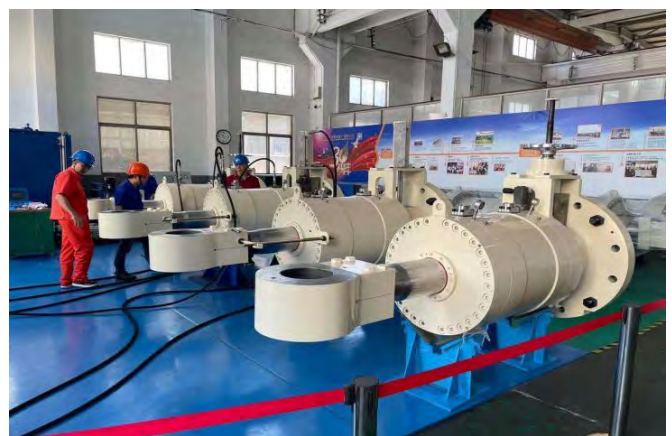
阳江导叶接力器 Guide vane servomotor of Yangjiang pumped-storage power station
