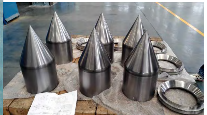
米纳斯水电站水轮机组喷针和口环过流表面热喷涂 Thermal spraying of needle and orifice ring overflow surface of water turbine unit of Minas Hydropower Station
