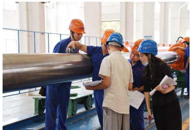
黄金峡水利枢纽工程 AP30 白陶涂层 AP30 white ceramic coating for the Huangjinxia Water Control Project
