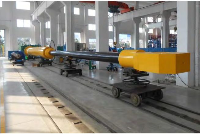
赞比亚伊泰兹水电站 AP20 黑陶涂层 Hydraulic system of Yangfanggou Hydropower Station
