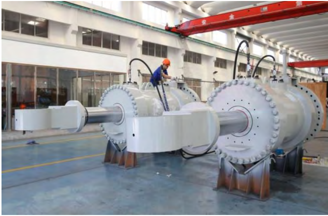
乌东德水电站水轮机组接力器, 单机容量 85 万千瓦 Hydroturbine unit servomotor of Wudongde Hydropower Station, with a unit capacity of 850000 kW
