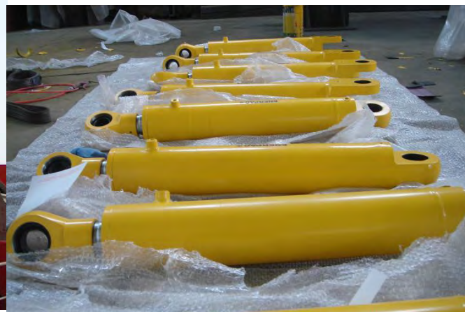
架桥机油缸 Bridge erecting machine oil cylinder
