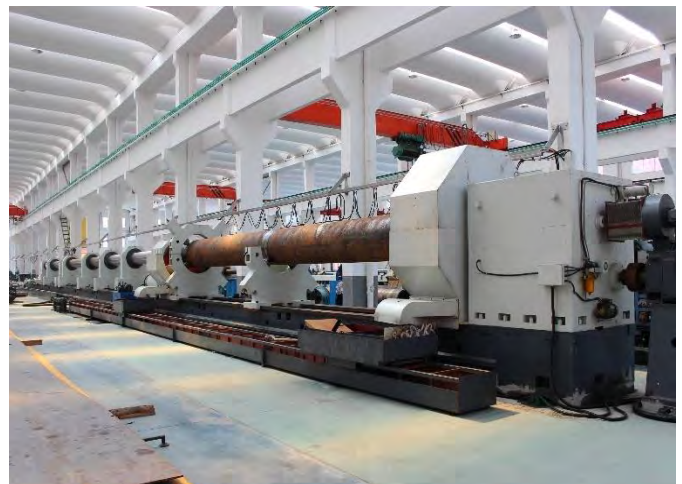
重型深孔镗床内孔直径 1.8m 长度 60m Heavy-duty deep hole boring machine, inner bore diameter 1.8m, length 60m
