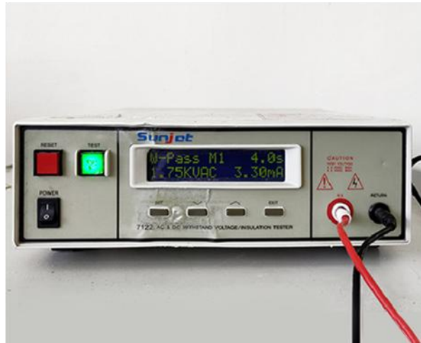
Power Withstand Voltage Test
