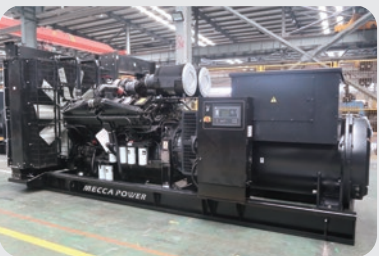
• Mining: 2 Units 1500KW Cummins Diesel Generator Sets
