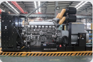
• Data Center: High Voltage 2500KVA Mitsubishi Generators
