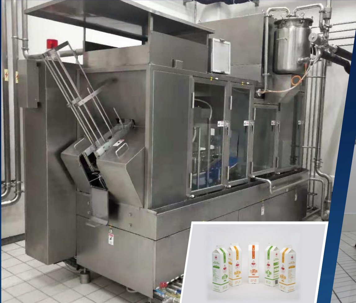
Gable-Top (Milk Carton) Filling Equipment
