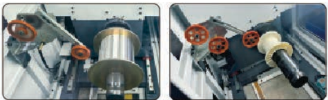
线盘尺寸 Bobbin Size 250-630mm (内孔Bore:127mm)
