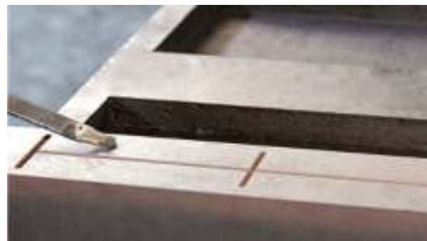
机床导轨运动面进行精密铲配合 Machine Tool's Motion Surface Experiences Precise Scraping
