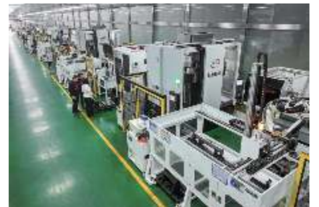
2023 第三代生产线 (可对接ETV小车、激光打码、数据上传) 2023 Third Generation Production Line (ETV Cart Dockable, Laser Coding, Data Upload)
