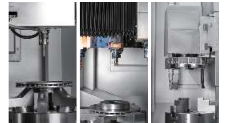
刹车盘专用结构 Brake Disc Specialized Structures 自动机内闭环检测补偿功能 Closed-loop Detection and Compensation Function Within The Automatic Machine 40/45/63硬导轨设计(针对淬火硬度50度以上零件加工) 40/45/63 Hard Rail (>50 HRC)
