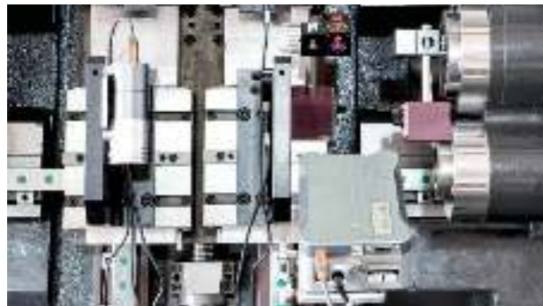
英国雷尼绍XL-80型激光干涉仪对机床的运动精度进行精密检测 Uk Renishaw XL-80 Laser Interferometer is Used To Precisely Test The Machine Tool's Motion Precision
