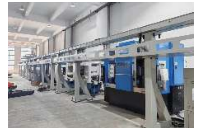
2024 第四代生产线 (自动监测、自动补偿) (自动换刀、产品柔性切换, 该功能正在测试中) 2024 Fourth Generation Production Line (Automatic Monitoring, Automatic Compensation)(Automatic Tool Change, Flexible Product Switching, This Function Is Under Testing)
