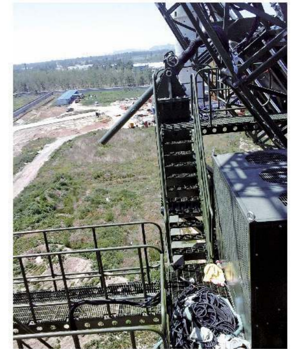
电动推杆用于俯仰设备 linear actuator rod for pitching equipment
