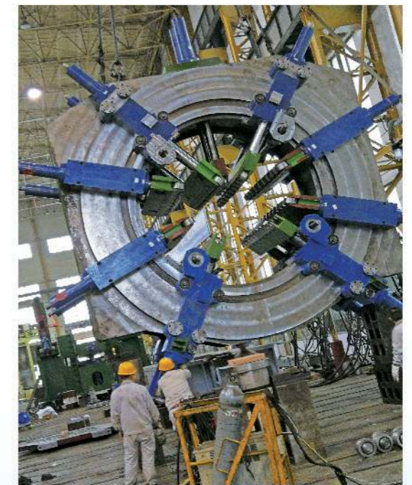
大型丝杆升降机用于螺旋焊管机 Application of large lifting Mechanism in Spiral welded Pipe Machine
